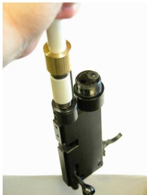
When you re-assemble the D12 air bushing you shall adjust this so that there is 2mm from the Front edge of the cocking slot and the cocking bolt, see picture.
