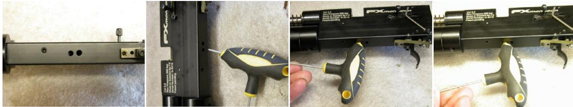
When shroud is removed it can be hard to remove D12, you might need to hit it with a plastic hammer.
