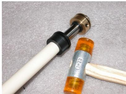
There will probably be marks on the barrel from the three screws holding it, grind these down.
